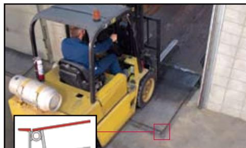
Traditional dock levellers have a gap at the rear hinge that creates a significant bump for fork-lift operators.
